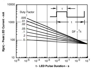
Figure 5. Maximum LED power dissipation
